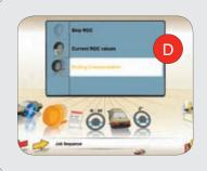
«RUN-OUT» COMPENSATION PROGRAM: Program to compensate «Run-Out» problems on tyre and rim and possible mistakes caused by an incorrect coupling between rim and self-centering clamp. The compensation value is calculated by pushing the vehicle for a distance corresponding to a wheel rotation of only 30°.
